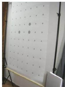
Fig. 4: Panel with holes placed at calibrated distances
